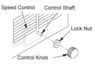
Figure 10 - Attaching Speed Control
